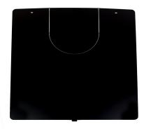
*NOTE:* The rear heat shield is designed to reduce the required clearance to a combustible surface behind the stove from behind the stove from 14" minimum to a 6" minimum. Please keep in mind that these clearances are **minimum** distances allowed.
